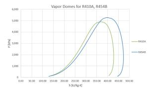
· 20% lower suction density for reduced mass flow rate
