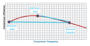
Figure 3: Conventional Part-load Control
