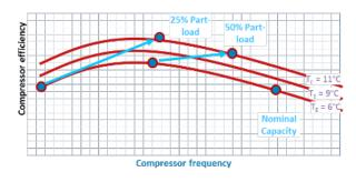
Figure 4: Part-load Operation with Increased Evaporator Temp
