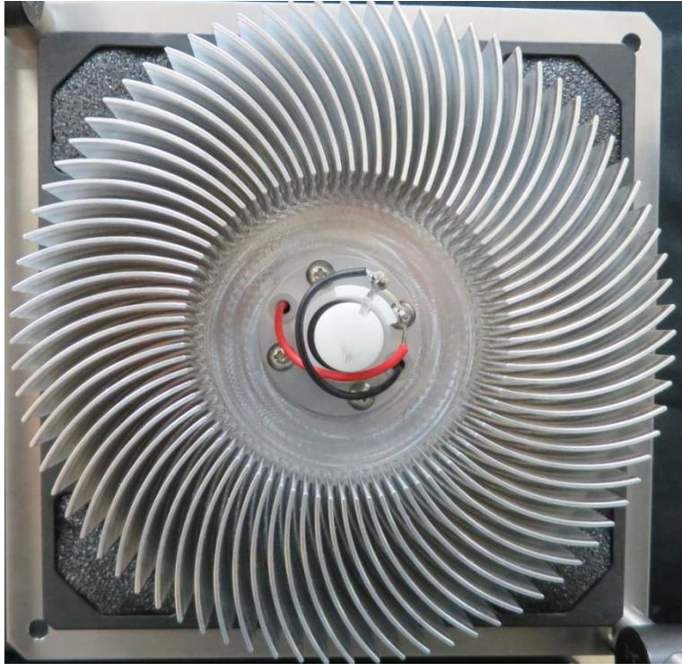
**Figure 35.** View of the cold side of the final assembly
