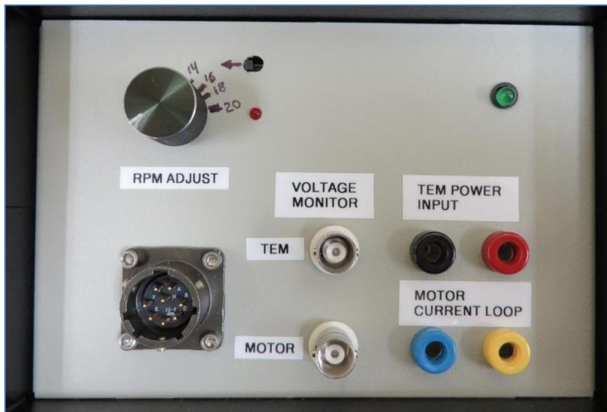
Figure 28. Control module front panel
