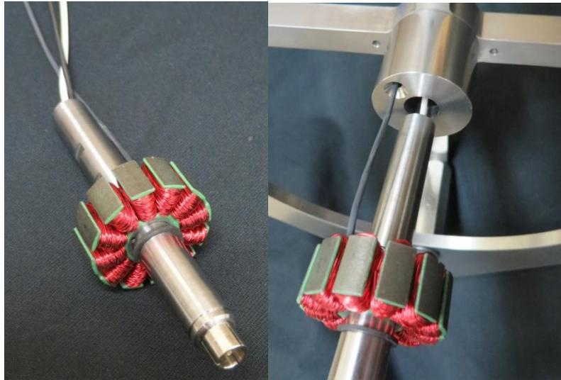
**Figure 29. Motor stator and shaft**
