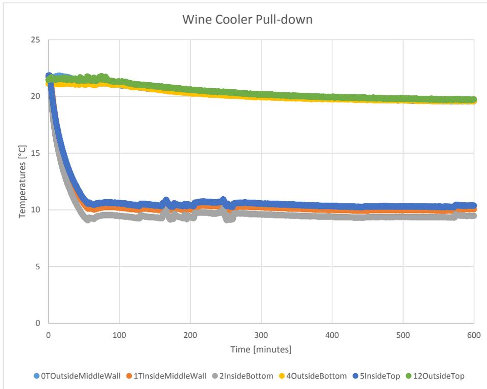
**Figure 9.** Pull-down time for baseline wine cooler, maximum  $\Delta T$  case
