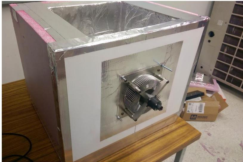
**Figure 42.** Improved enclosure insulation
